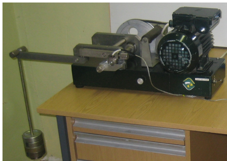
Fig. 2. General view of the modernized Timken-Machine friction machine
